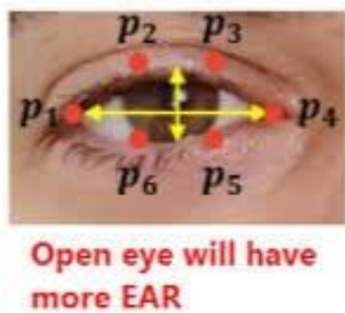
Figure 9. In this figure, the study of eyes P1, P2, P3, P4, P5, and P6 used to measure the eye-to-eye ratio (EAR) with eyes open is approximately 0.24.
